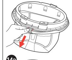
14D. Remove the edge of the Seat Fabric from the Seat Frame.
