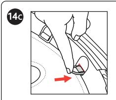
14C. While pushing the ring through the opening on the Seat Frame, at the same time, pull the strap from the opposite side of the opening. Next, remove both rings on either side of the first ring. Alternate removing a ring from each side until you have removed all of the rings.
