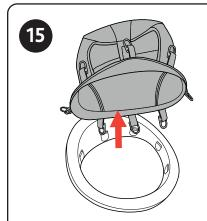
15. Remove the fabric seat covering from the Seat Frame, as shown.
