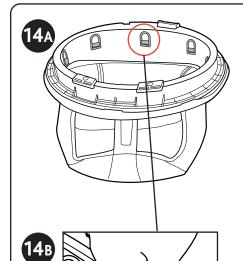
14A. Locate 8 plastic rings on the inside of the Seat Frame.
